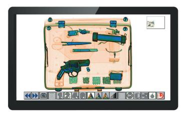
L-3's operator interface is a touch screen that allows continuous heads-up operation using icons displayed on the viewing screen
